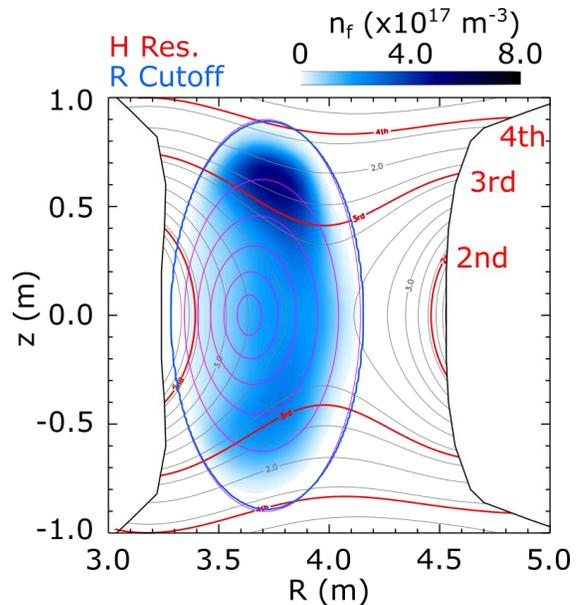
FIG. 2. The lines are calculated flux and magnetic field contour, right hand cutoff, and the hydrogen resonance layer of the ICRF heating in the condition of 100% hydrogen, magnetic field of 1 T and  $k_{\parallel}=5.0 \text{ m}^{-1}$ . The blue color contour is energetic particle flux density supplied by 40 kV radial NBIs. This flux density is calculated by MORH code.
