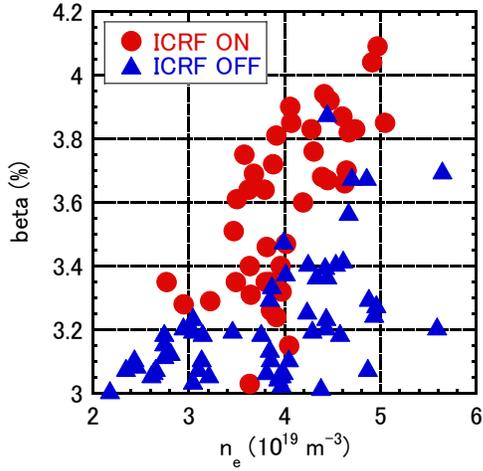
FIG. 3. The achieved beta value of all the discharges of high beta experiment in LHD 18th campaign in 2014-15. The ICRF heating clearly contributed to the increase of beta value.
