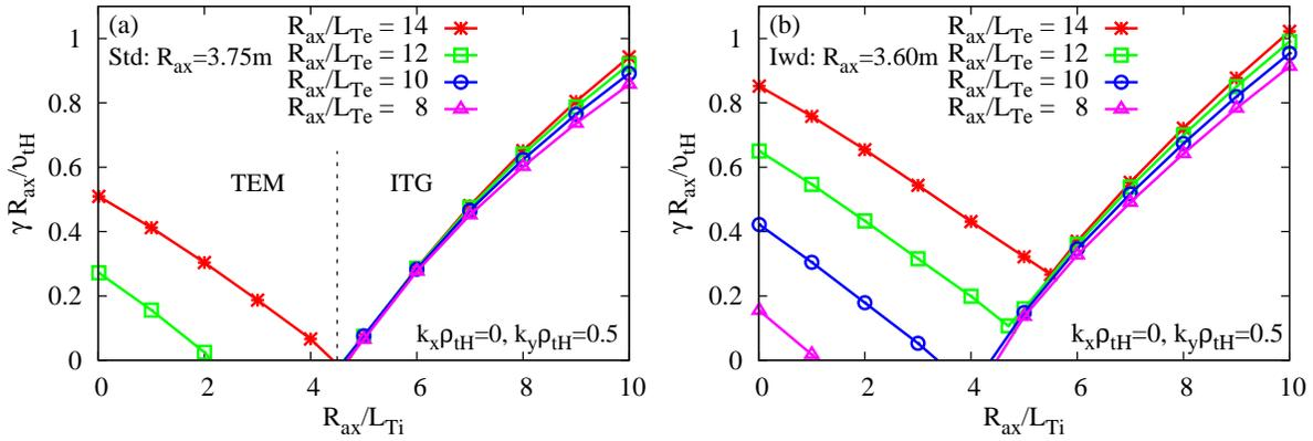
**Figure 2.** ITG and TEM growth rates in the hydrogen( $s=H$ ) helical plasma with (a)the standard and (b)inward-shifted configurations, where  $R_{ax}/L_n=2$ ,  $T_e/T_i=2$ , and  $\nu_{ei}^* \simeq 0.04$  are fixed.
