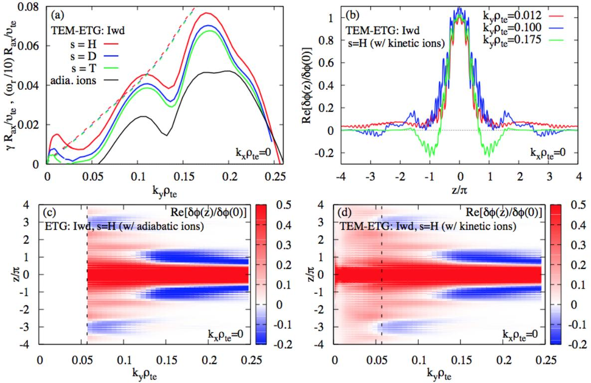
**Figure 5.** (a) The growth rate (solid) and the mode frequency (dashed) in ETG modes, (b) the real part of eigen-mode structures in the field-line direction  $z$ , and the  $(k_y, z)$ -contour map of the real part of eigen-modes for (c) adiabatic-ion and (d) kinetic-ion cases.
