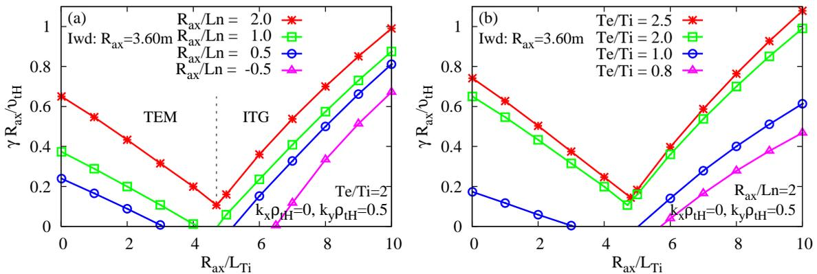
**Figure 3.** Parameter dependence of (a)the density gradient  $R_{ax}/L_n$  and (b)the temperature ratio  $T_e/T_i$  on the ITG and TEM growth rates, where  $R_{ax}/L_{T_e} = 12$  and  $\nu_{ei}^* \simeq 0.04$  are fixed.
