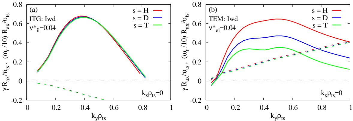
**Figure 4.** Comparison of the normalized linear growth rate  $\gamma R_{ax}/v_{ts}$  (solid) and mode frequency  $\omega_r R_{ax}/v_{ts}$  (dashed) in (a)ITG and (b)TEM instabilities with the hydrogen isotope species.
