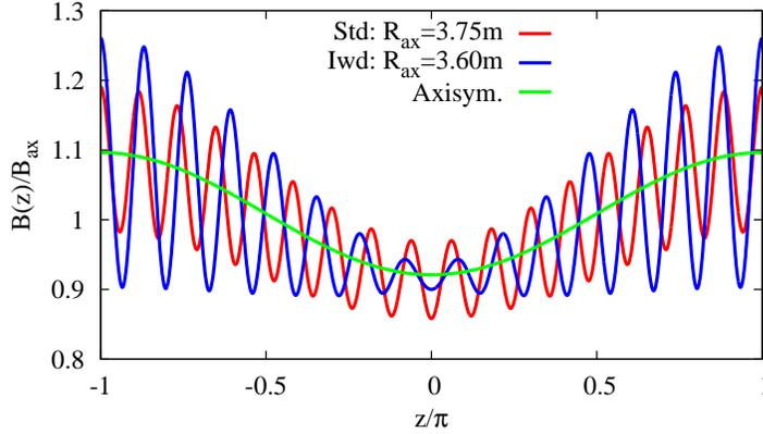
**Figure 1.** Magnetic field intensity along the field line for the standard (Std:  $R_{ax} = 3.75\text{m}$ ) and the inward-shifted (Iwd:  $R_{ax} = 3.60\text{m}$ ) plasma configurations, where the axisymmetric case is also plotted for comparison.
