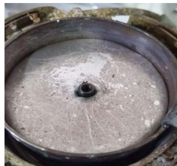
Fig. 4 The surface of \text{Ga}_{67}\text{In}_{20.5}\text{Sn}_{12.5} after plasma exposure, showing a buoying contamination film.
