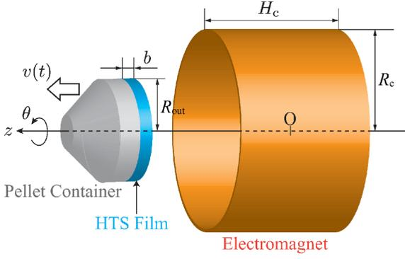
Fig. 8. A schematic view of the SLA system.
