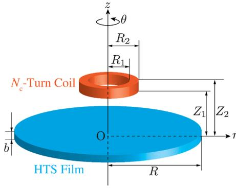
Fig. 5. A schematic view of the inductive method.
