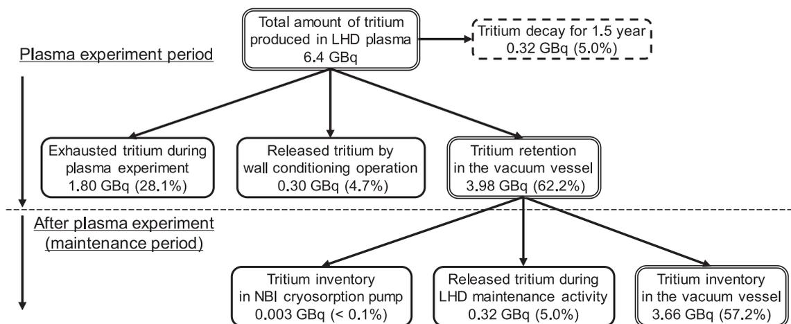
Fig. 8 The diagram of tritium balance in LHD throughout the first deuterium plasma experiment campaign and the maintenance activity.
