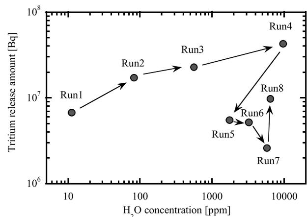
Fig. 3 The dependence of the water vapor concentration on the tritium release amount from the LHD vacuum vessel at room temperature.
