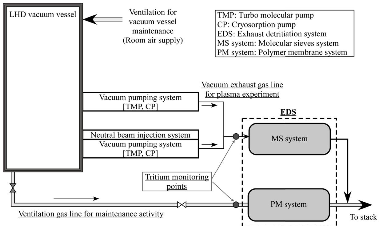
Fig. 1 A schematic of the system of the LHD vacuum exhaust and the air ventilation during the maintenance activity.
