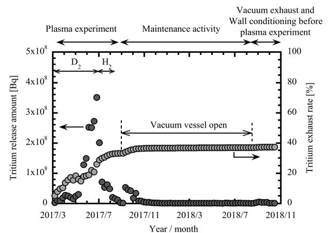
Fig. 6 The variation of the exhausted tritium amount and the exhausted tritium rate during the first deuterium plasma experiment campaign and the maintenance activity.
