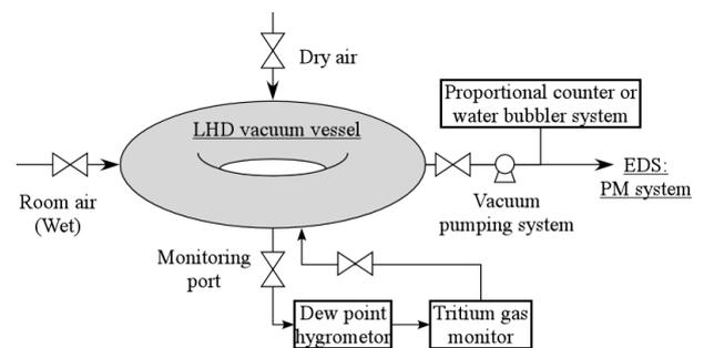
Fig. 2 The schematic diagram of the configuration for the experiment on tritium release from the LHD vacuum vessel.
