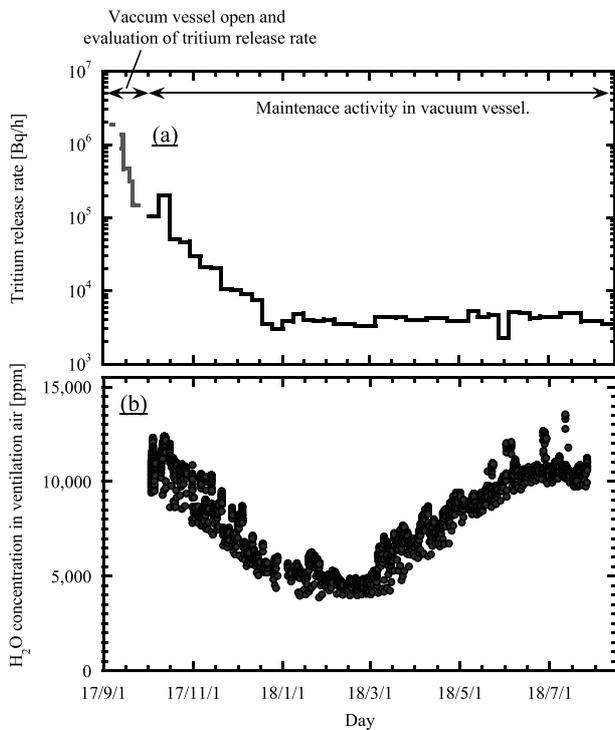
Fig. 5 The variations of the tritium release rate and water vapor concentration in the ventilation air during the LHD vacuum vessel maintenance activity: (a) tritium release rate, (b) water vapor concentration.
