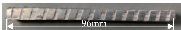
Fig. 1 Overview of the short sample of the conductor consisting of stacked YBCO tapes without twist. YBCO tapes were fabricated by SuperOx. The number of tapes in the conductor was 50. The conductor was spirally wrapped in a copper sheet.
