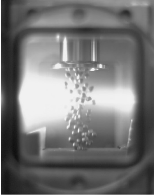
Figure 7 The photo of the plasma with the pebble flow taken by a high-speed camera (shutter speed: 1/1,000 sec). The left side of the photo corresponds to the plasma upstream.
