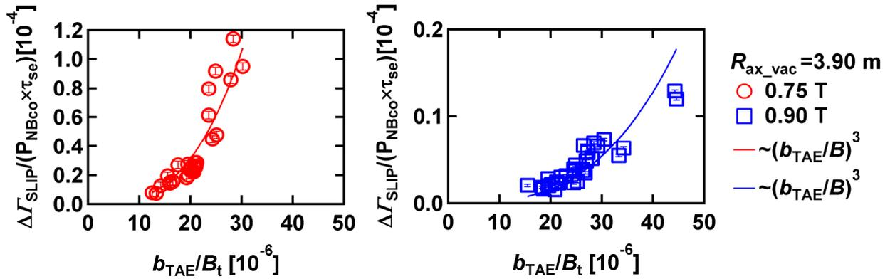
Fig. 3 Dependence of the normalized lost fast-ion flux induced by TAE on the magnetic fluctuation amplitude of TAE. The normalized loss flux on  $B_t = 0.75 \text{ T}$  and  $0.90 \text{ T}$  are scaled with  $(b_{\text{TAE}}/B_t)^3$ .
