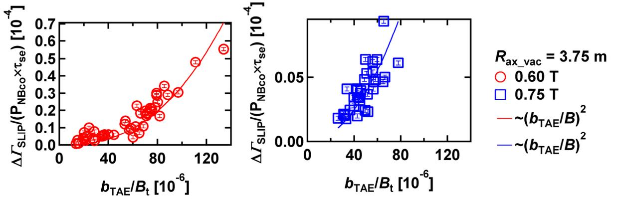
Fig. 2 Dependence of the normalized lost fast-ion flux induced by TAE on the magnetic fluctuation amplitude of TAE. The normalized loss fluxes at  $B_t = 0.60 \text{ T}$  and  $0.75 \text{ T}$  are scaled with  $(b_{\text{TAE}}/B_t)^2$ .
