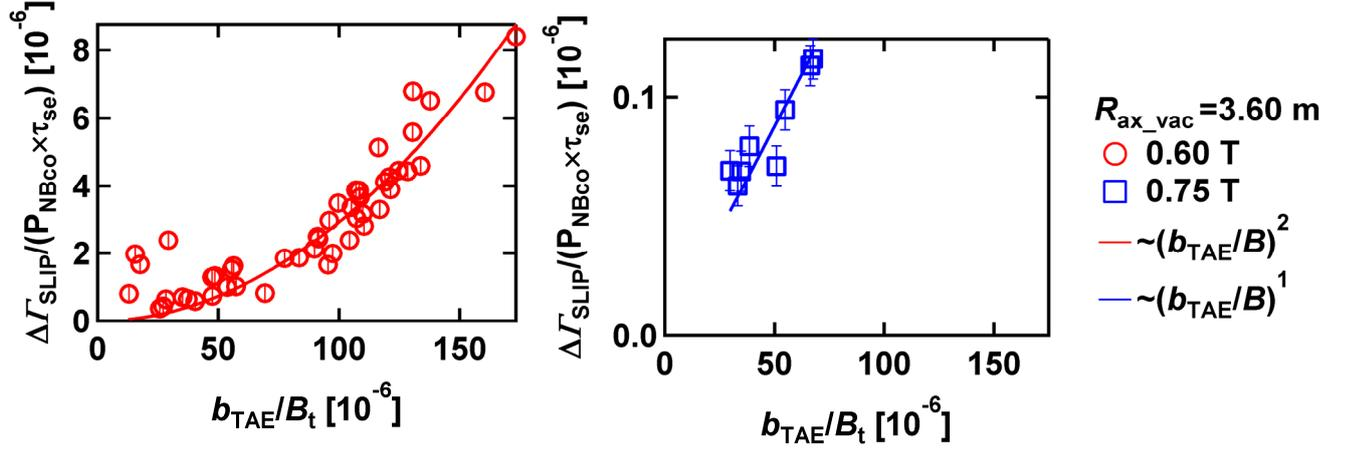
Fig. 1 Dependence of the normalized lost fast-ion fluxes on the magnetic fluctuation amplitude of TAE. The loss fluxes at  $B_t = 0.60 \text{ T}$  and  $0.75 \text{ T}$  are respectively scaled with  $(b_{\text{TAE}}/B_t)^2$  and  $(b_{\text{TAE}}/B_t)^1$ .
