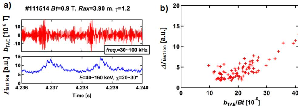
Fig. 4 a) Typical time traces of magnetic fluctuation of a TAE range of frequency and signal of lost-fast ion ( $b_{TAE}$ ). b) Increment of fast-ion loss as a function of TAE amplitude measured at magnetic probe position normalized by toroidal magnetic field strength. Increment of fast-ion loss increase with TAE amplitude.
