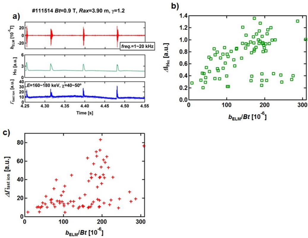
Fig. 5 a) Typical time traces of magnetic fluctuation of ELM range of frequency,  $H\alpha$  signal, and signal of lost-fast ion. b) Increment of  $H\alpha$  signal as a function of ELM amplitude measured at magnetic probe position ( $b_{ELM}$ ) normalized by toroidal magnetic field strength. There are no clear dependence. c) Increment of fast-ion loss as a function of  $b_{ELM}/Bt$ . It has a dispersed structure.
