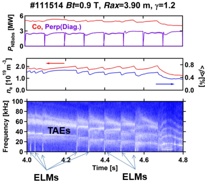
Fig. 3 Time trace of absorbed power of neutral beam injection ( $P_{NBabs}$ ) of NB1 and diagnostic beams, line averaged density, volume averaged beta and power spectrogram of Mirnov signal on typical discharge with TAEs and ELMs.
