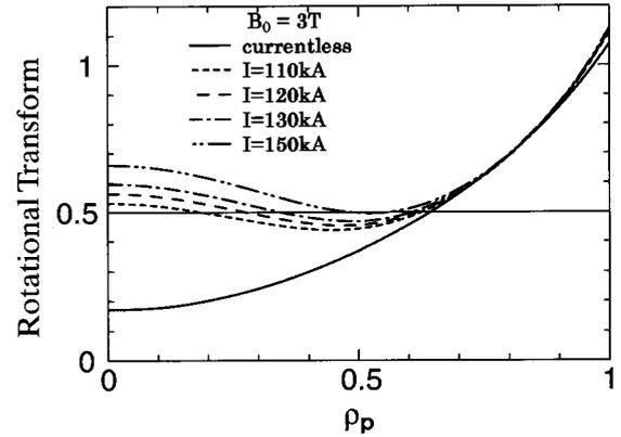
Fig. 1 Profiles of the rotational transform for the various net toroidal currents. The radius  $\rho_p$  denotes the square root of the normalized equilibrium poloidal flux, which is also used in Figs. 3, 5 and 6.
