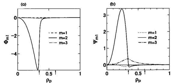
Fig. 3 Mode structures of (a) stream function and (b) poloidal flux of the  $n = 1$  ideal internal kink mode for  $I = 130 \text{ kA}$ . The arrows indicate the positions of  $\iota = 1/2$  surfaces, which are also used in Figs. 5 and 6.
