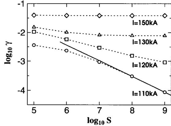
Fig. 4  $S$ -Dependence of the growth rate of the  $n = 1$  resistive mode. Solid line shows the dependence determined with  $\gamma(S = 10^8)$  and  $\gamma(S = 10^9)$ , which corresponds to  $\gamma \propto S^{-0.54}$ .
