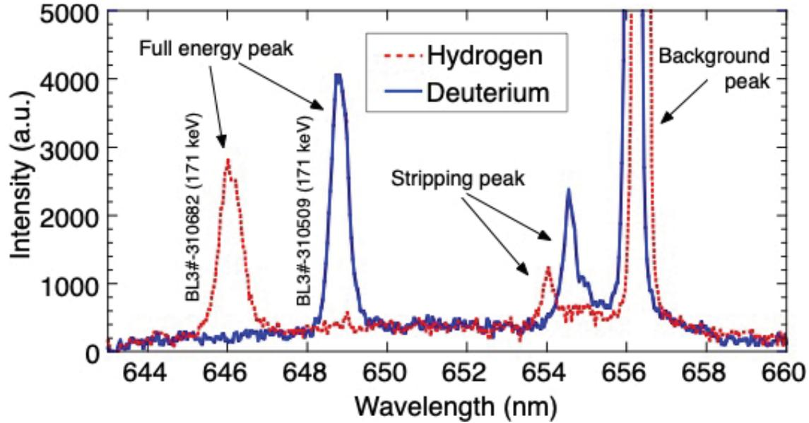
**FIGURE 2.** The Doppler shifted beam emission spectra of hydrogen (dotted line) and deuterium (bold line) appear on the blueshift side of the non-shifted background spectrum from the ion source. The peaks from full energy (171 keV) beam and stripping neutrals on the low energy position are observed.
