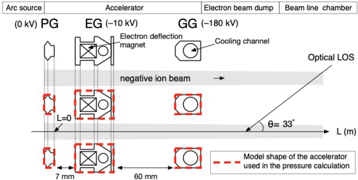
**FIGURE 1.** The cross-sectional drawing of the beam accelerator of the negative ion source in the N-NBI (BL3) in LHD. The optical line of sight to observed beam emission  $H_\alpha$  is set  $33^\circ$  to the center of beam line.
