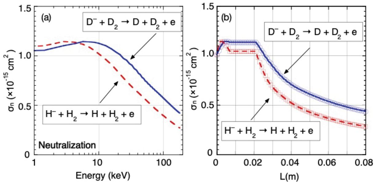
**FIGURE 4.** Energy distribution (a) and spatial distribution (b) of the neutralization cross-sections of hydrogen (dashed line) and deuterium (bold line) inside the accelerator. The reaction cross-section is referred from the Oak Ridge National Laboratory database [14]
