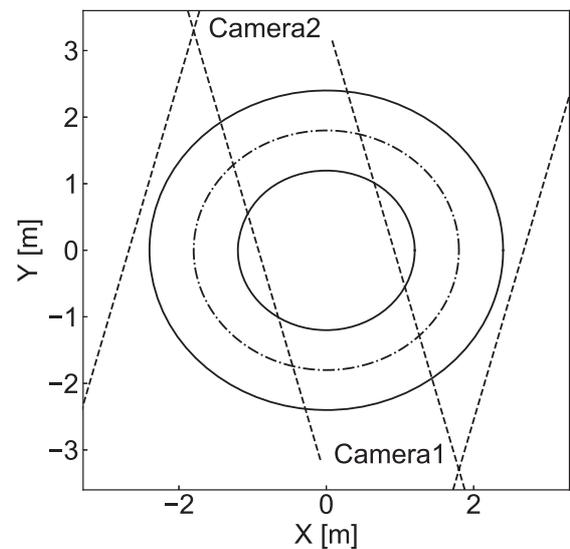
Fig. 4 Schematic drawing of the camera system for testing the tangentially viewing imaging system. It is noted that the center of the sight line is on the equatorial plane.
