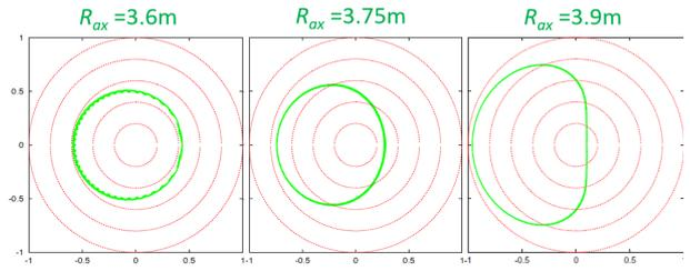
Fig. 5 Collisionless orbits of helically trapped energetic ions in  $R_{ax}$  of 3.6 m, 3.75 m, and 3.9 m.
