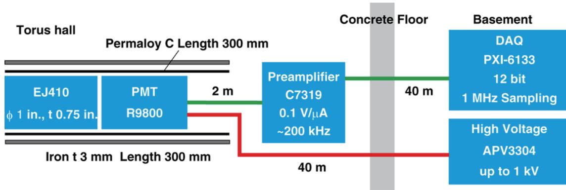
Fig. 1 Block diagram for fast-neutron scintillation diagnostics.
