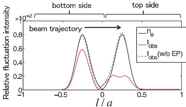
Fig. 2 Comparison of the density fluctuation with the simulated signal of HIBP in the case of  $\alpha = 3$ . Electron density fluctuation, simulated signal with and without the fast ion effect are shown by the black, blue and magenta lines, respectively.
