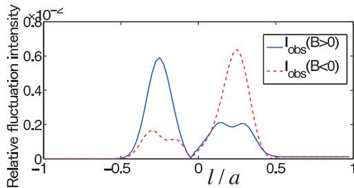
Fig. 4 Simulated signals of HIBP in the case of  $\alpha = 3$  for the positive and negative magnetic fields.
