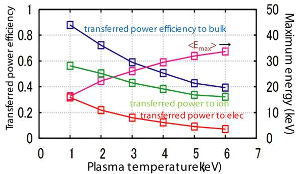
Fig. 6 Temperature dependence of transferred power efficiency with  $n_e = 1.0 \times 10^{19} \text{ m}^{-3}$ .
