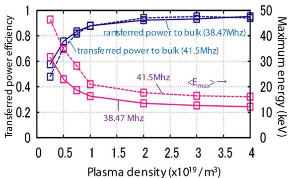
Fig. 9 Difference of transferred power efficiency and maximum energy due to position of resonance layer with  $T_e = 1$  keV.
