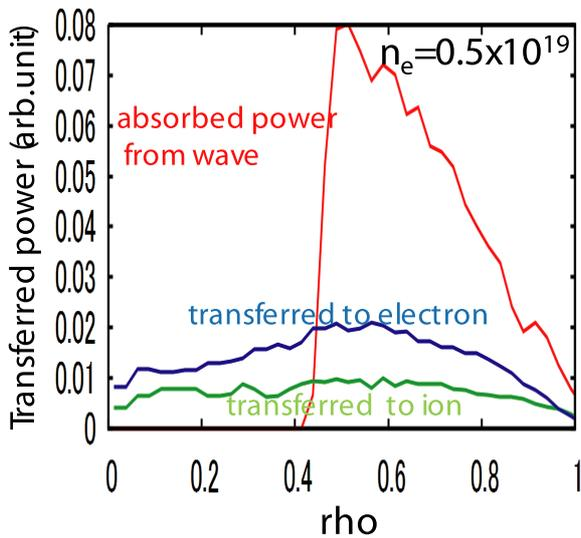
Fig. 4 Typical profiles of the transferred power and absorbed power from wave in the case of  $T_e = 1$  keV and  $n_e = 0.5 \times 10^{19} \text{ m}^{-3}$ .
