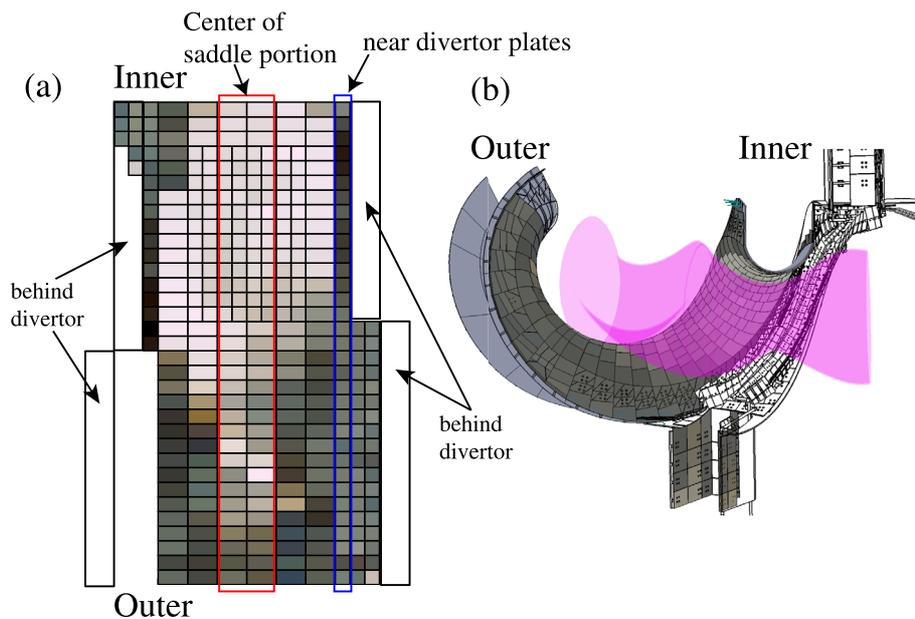
Fig. 2 (a) Developed view and (b) CAD showing the color distribution of the measured stainless steel plates. A typical plasma shape is drawn in (b).
