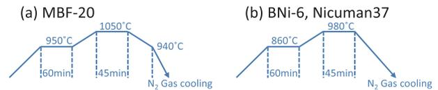
Fig. 2 Procedures of the heat treatment of (a) MBF-20 and (b) BNI-6 and Nicuman37 filler materials.
