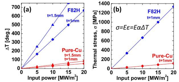
Fig. 1 (a) Temperature gradient as a function of an input power in different thickness of F82H ( $30 \text{ W/m}\cdot\text{K}$ ) and Pure-Cu ( $320 \text{ W/m}\cdot\text{K}$ ). (b) Induced internal thermal stress ( $\sigma$ ) as a function of an input power in the 1 mm thickness of F82H and Pure-Cu.  $E$ : Young’s modulus [Pa],  $\alpha$ : Thermal expansion coefficient [ $\text{K}^{-1}$ ].
