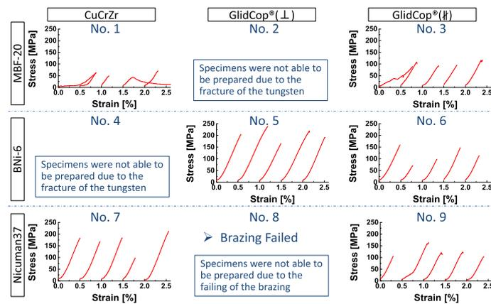
Fig. 3 Stress-strain curve of the three point bending test for the nine combination patterns of the copper alloys and the filler materials.
