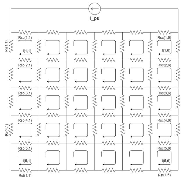
Fig. 2 2D resistor grid for 5 HTS tapes. The top 5 rows correspond to superconducting resistance segments of each HTS tape ( $R_{sc}$ ); last row is the stabilizer equivalent resistance ( $R_{sr}$ ); and vertical resistances account for the contact resistance between each tape superconducting layer ( $R_v$ ).
