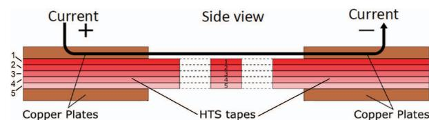
Fig. 1 Schematic of the experimental setup, to produce a non-uniform current distribution in a stack of HTS tapes. Injecting the current from one edge of the stack produces the worst-case scenario. From [4].
