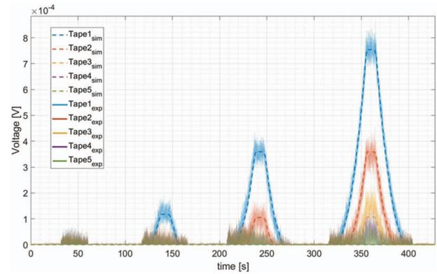
Fig. 5 Voltage comparison between experimental data (continuous lines) and simulation (dashed lines). Critical current adjustment and experimental contact resistance leads to a reasonably good match.
