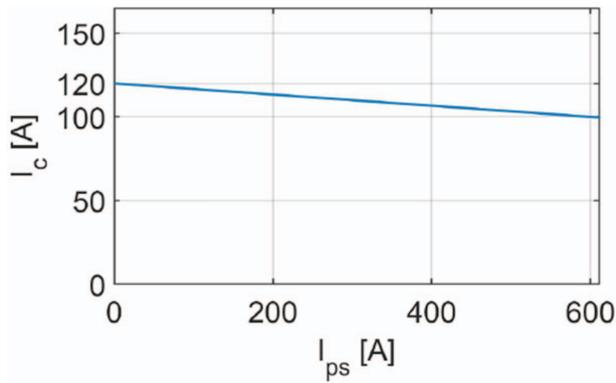
Fig. 4 Linear decreasing trend for critical current ( $I_c$ ) as function of the total input current ( $I_{ps}$ ), for one HTS tape.
