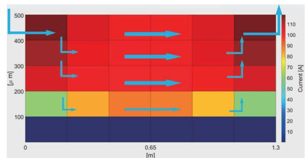
Fig. 6 Current distribution in each superconducting segment for 400 [A]. The color of each square is the horizontal current flowing through it, and the blue arrows are indications of how there is a current share at bottom tapes.
