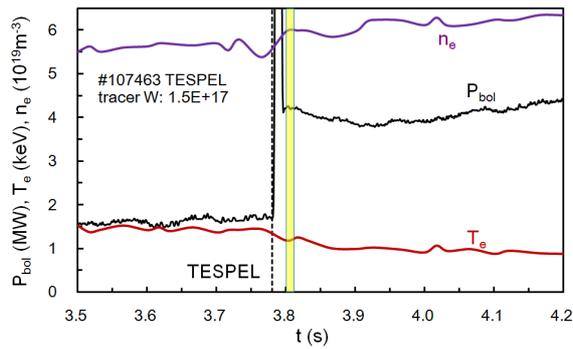
Fig. 1 Temporal developments of  $P_{\text{bol}}$  and the local value of  $T_e$  and  $n_e$  at  $r_{\text{eff}} = 0.40$  m. The TESPEL having the tungsten tracer is injected at the timing denoted by the dotted line.
