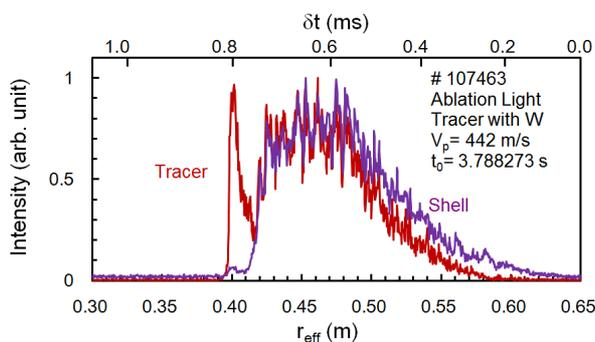
Fig. 2 Temporal developments and corresponding locations of the ablation light emissions through the filters for the shell and the tracer, respectively.  $\delta t$  stands for the time passed after the time  $t_0$ .
