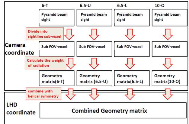
Fig. 2 Flowchart of geometry matrix calculation.
