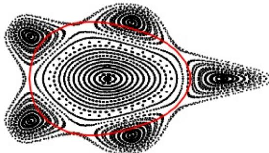
Figure 3 Magnetic configuration of island bundle divertor.
