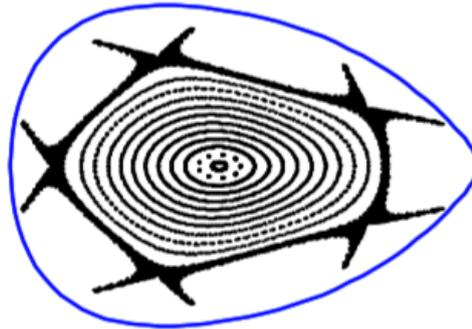
Figure 5 Divertor field line tracing with assumed existence of divertor targets.
