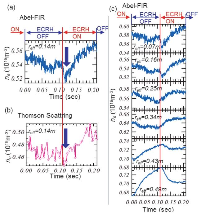
Fig. 6 Temporal evolution of electron density measured by (a) Abel-FIR and (b) TS near the heating position. (c) Electron density measured by Abel-FIR at each position. Heating position is  $r_{\text{eff}} \sim 0.19\text{m}$ .
