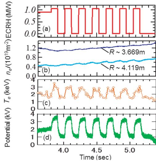
Fig. 3 Temporal evolution of (a) ECRH injection power, (b) line-integrated electron density from the upper to lower trace at  $R = 3.669$  and  $4.119$  m measured by FIR laser interferometers, (c) electron temperature and (d) electric potential near the heating position ( $r_{\text{eff}} \sim 0.19$  m). Magnetic axis  $R_{\text{ax}}$  is 3.6 m. Minor radius  $a_{99}$  is 0.6 m.
