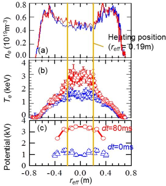
Fig. 4 Profiles of (a) electron density measured by TS, (b) electron temperature and (c) electric potential before ECRH injection (blue,  $dt = 0\text{ms}$ ) and 80 ms after ECRH injection (red,  $dt = 80\text{ms}$ ).
