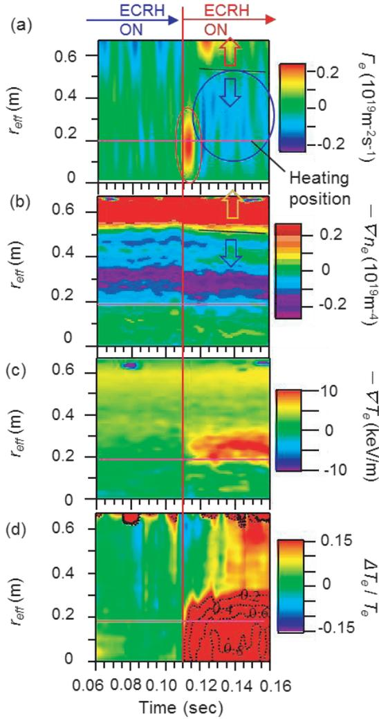
Fig. 8 (a) Electron flux estimated by Abel-FIR. (b)  $-\nabla n_e$ , (c)  $-\nabla T_e$  estimated with  $n_e$ ,  $T_e$  measured by TS. (d) Electron temperature increment ratio to that just after ECRH injection.
