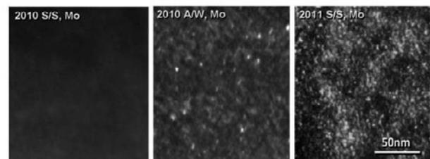
Fig.2 Formation of dislocation loops in Mo placed at equator part in the campaigns of 2010S/S, 2010A/W and 2011S/S.
