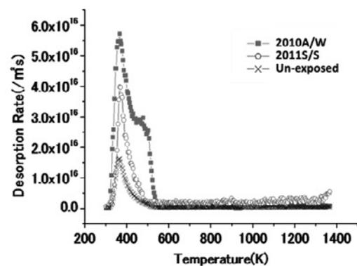
Fig.3 TDS spectrum of implanted deuterium from W exposed to plasmas in 2010A/W and 2011S/S.
