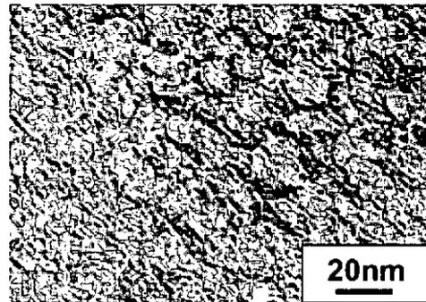
Fig. 1 TEM image of tungsten exposed to helium discharge cleaning
