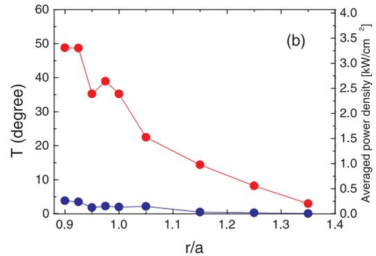
Fig. 4 (a) The time trace of probe head temperature, and (b) the temperature increase as a function normalized minor radius.
