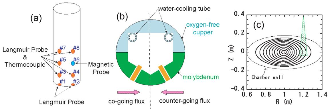
Fig. 1 Schematics of (a) the probe array on the hybrid directional probe, (b) cross-section of the HDP, and (c) the magnetic surface of outward-shifted configuration with  $R_{ax} = 0.974$  m and scannable area of the HDP in a horizontally elongated cross-section of CHS.
