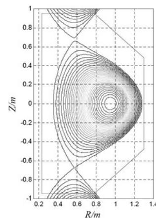
Fig. 2: OH divertor plasma of lower triangularity (Candy-shape) was produced with PF35-12 and reconstructed by Windows E-FIT.
