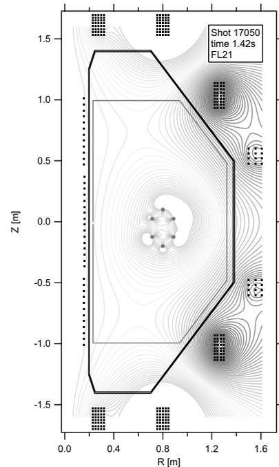
Fig. 1: OH divertor plasma of lower triangularity (Candy-shape) produced with PF35-12 and reconstructed by QUEST CCS.
