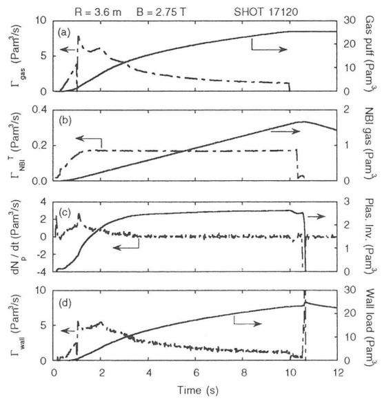
Fig. 1 Particle balance for hydrogen discharge: (a) gas puff, (b) fueling by NBI, (c) plasma inventory, (d) inferred wall load.
