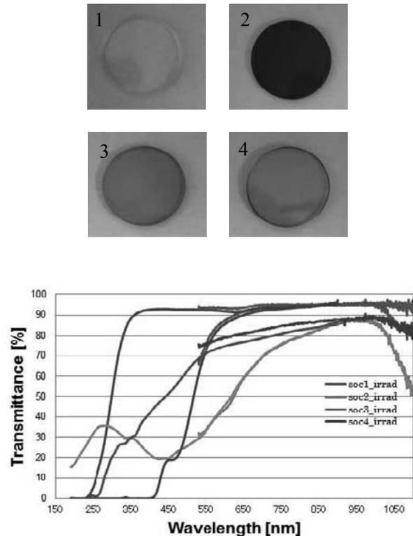
Fig.1 Transmittance of samples SOC-1, 2, 3, and 4 after JRR-3 irradiation (48 hours, 22K2009).
