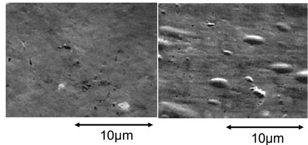
Figure 1 SEM images of surface morphology of W irradiated with pre-irradiated He fluence of (a)  $1 \times 10^{17}$  He/cm<sup>2</sup> and (b)  $1 \times 10^{18}$  He/cm<sup>2</sup>.
