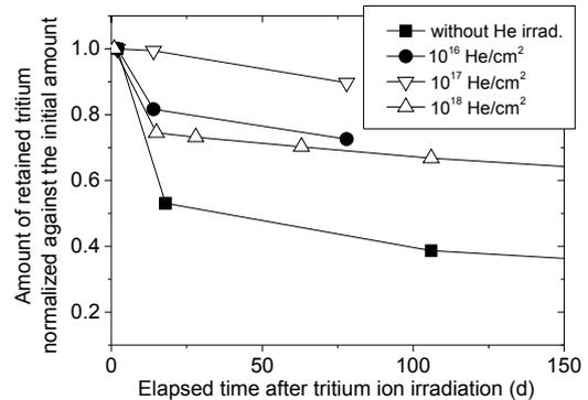
Figure 3 Time evolution of amount of retained T for He pre-irradiated W during preservation in vacuum.
