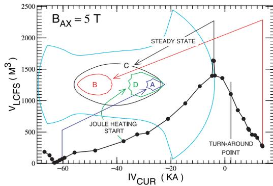
Fig. 2 Variation of the volume and shape of the last closed magnetic surface with the IV coil (2880 turns) current sweep. The magnetic surface “D” is the initial magnetic surface before Joule heating. The magnetic surface “C” is the steady-state magnetic surface after terminating Joule heating. The turn-around point of the IV coil current is also shown.
