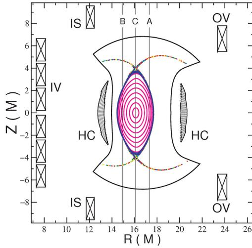
Fig. 1 An example of coil systems and machine size for a DT reactor. A Poincaré plot of the lines of force for an optimized magnetic surface, similarity expanded vacuum vessel of the LHD, cross sections of the helical coils (HC) and the vertical field coils (IV, IS, OV) are shown. The position of the magnetic axis can be shifted from “A” to “C” by the IV coil current.
