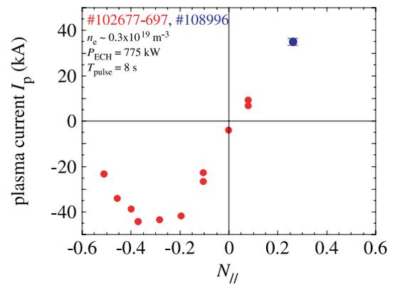
Fig. 5 Dependence of plasma current  $I_p$  at the end of the discharges (at 9 s) is plotted as a function of EC-wave beam direction  $N_{||}$ . The data point with  $N_{||} = 0.27$  is an extrapolation from the discharge with 4 s duration.
