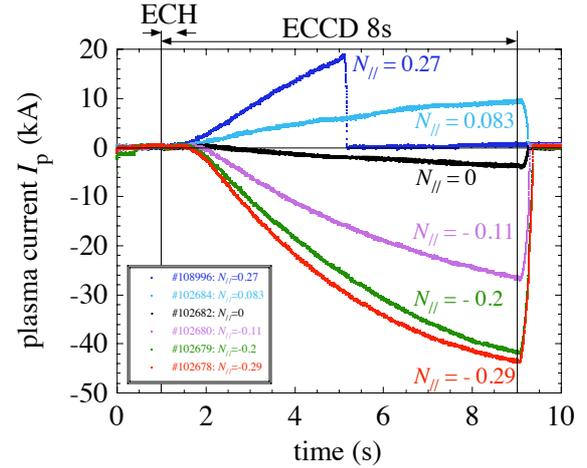
Fig. 4 Time evolutions of plasma current in the discharges with various EC-wave beam direction.
