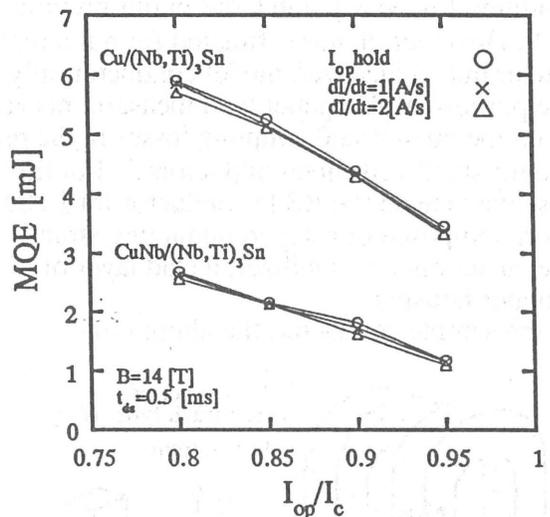
Fig. 2 Current and dI/dt dependence on both the Cu/(Nb,Ti)<sub>3</sub>Sn wire and the CuNb/(Nb,Ti)<sub>3</sub>Sn wire.
