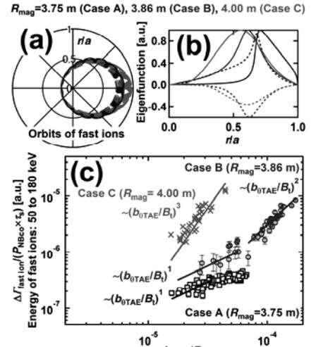
Fig. 1 (a) Co-circulating fast-ion orbits in cases A, B, and C on  $B_t=0.6\text{ T}$ . (b) Eigenfunctions of TAE calculated by AE3D for cases A, B, and C. (c)  $\Delta\Gamma_{\text{fast ion}}/(P_{\text{NBco}} \times \tau_s)$  as a function of  $b_{\theta\text{TAE}}/B_t$ . Dependence of fast-ion loss flux on simulation is shown in Fig. 2. In case B, the
