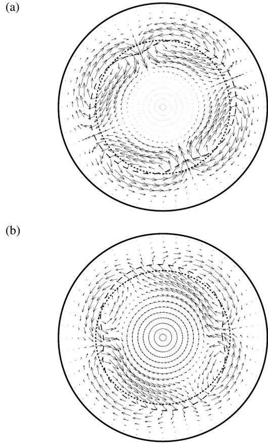
Fig. 2 Flow pattern at (a)  $t = 9,600\tau_A$  and (b)  $t = 18,000\tau_A$  for  $r \leq 0.8$ . Dotted and dashed lines show the position of the surfaces with  $\iota_T = 1/2$  and  $\iota_{eq} = 1/2$ , respectively.
