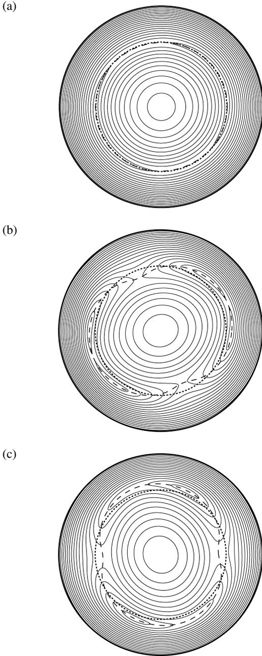
Fig. 3 Contour of  $\psi_h$  at (a)  $t = 3,000\tau_A$ , (b)  $t = 9,600\tau_A$  and (c)  $t = 18,000\tau_A$  for  $r \leq 0.8$ . Dotted and dashed lines show the position of the surfaces with  $\tau_r = 1/2$  and  $\tau_{eq} = 1/2$ , respectively.
