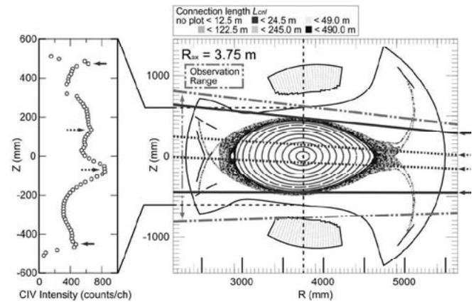
Fig. 1. The observation range of VUV spectroscopy shown on the poloidal cross section of LHD together with full vertical profile of line intensity of CIV 1548.20 × 2 Å spectrum.
