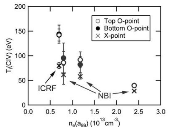
Fig. 2. Dependence of ion temperature  $T_i$  obtained from Dopplar broadening of CIV spectrum on edge electron density  $n_e(a_{99})$ .
