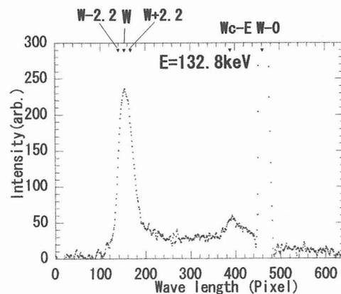
Fig.2 Energy spectrum of H<sub>0</sub> beam in LHD-NBI H<sup>-</sup> ion source
