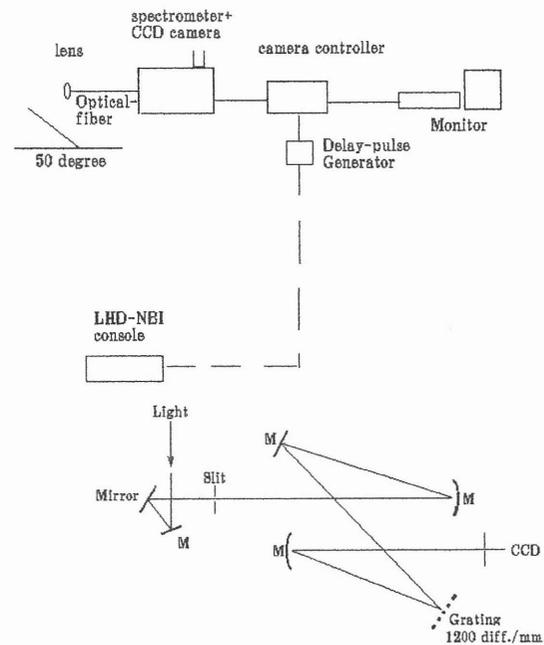
Fig.1 Doppler shift spectroscopy system (top) and grating-25cm spectrometer (bottom)
