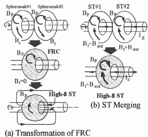
Fig. 1. Three types of high-beta ST formations: (a) transformation of FRC, (b) merging STs, (c) multiple ST merging, and (d) electrodeless merging using X-point ST formation.
