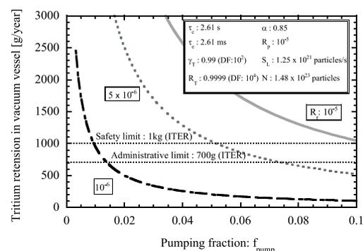
Fig. 5 Tritium retention in the vacuum vessel as the functions of pumping fraction and tritium loss ratio by retention in the vacuum vessel,  $R_T$ .
