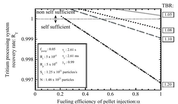
Fig. 2 The dependence of tritium recovery rate in the tritium processing system as a function of the fuel efficiency of pellet injection for FFHR2m2.
