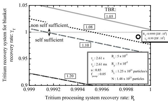
Fig. 3 Fuel self-sufficiency condition for FFHR DEMO reactor system as the functions of TBR and the recovery rate for tritium processing system, and tritium recovery system for blanket,  $R_T$  and  $\gamma_T$ .
