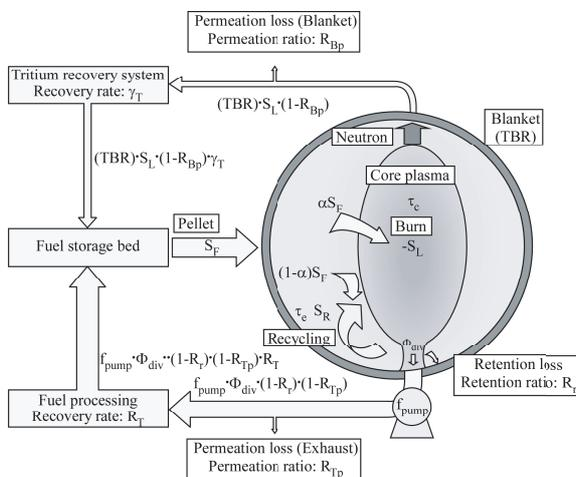
Fig. 1 Steady-state analytical model for calculating tritium balance in a fusion reactor.
