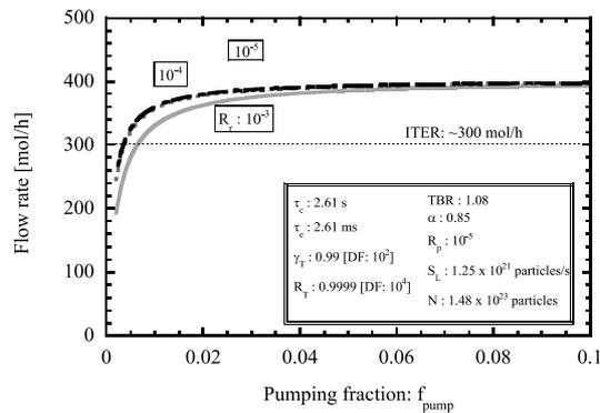
Fig. 6 The estimated flow rate from the vacuum vessel as the functions of pumping fraction and tritium loss ratio by retention in the vacuum vessel,  $R_r$ .
