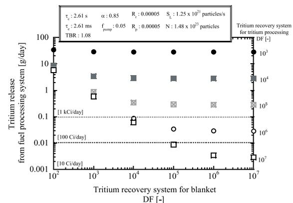
Fig. 4 Tritium loss from the tritium recovery system as the functions of decontamination factor for blanket system and tritium processing system for vacuum exhaust gas.
