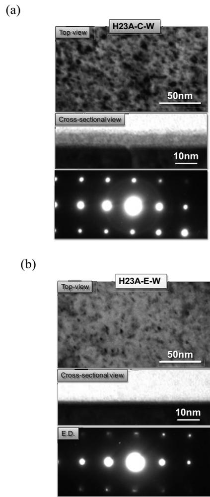
Fig. 3 Top view and cross-sectional view of TEM images, and electron diffraction pattern of (a) the thinned tungsten specimen that was set at the central position and (b) that at the east position.
