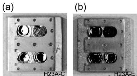
Fig.2 Sample holders with TEM specimens (a) at the central position indicated with “A” in Fig. 1 and (b) at the east position indicated with “B” in Fig. 1.
