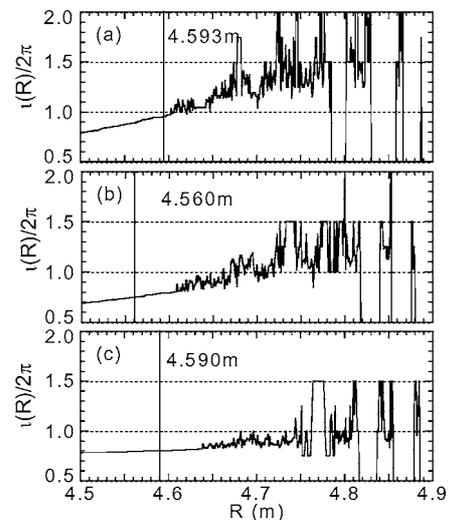
Fig. 1 Rotational transform in (a)  $R_{ax} = 3.90$  m, (b)  $4.00$  m and (c)  $4.10$  m. Solid lines show LCFS position.
