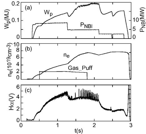
Fig. 2 H-mode-like discharge obtained in  $R_{ax} = 4.00$  m configuration; (a) plasma stored energy and NBI power, (b) density and (c)  $H_{\alpha}$  signal.
