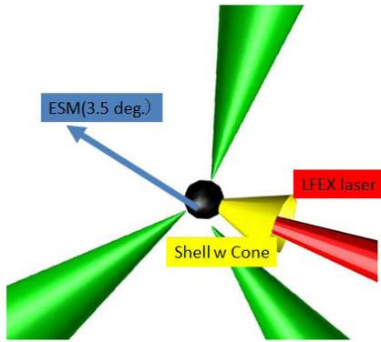
Fig. 1 Experimental setup. Shell with cone is imploded by the green laser. Imploded core is auxiliary heated by the hot electron created by the interaction between the LFEX laser and the cone tip. Escaped hot electrons are measured by ESM.
