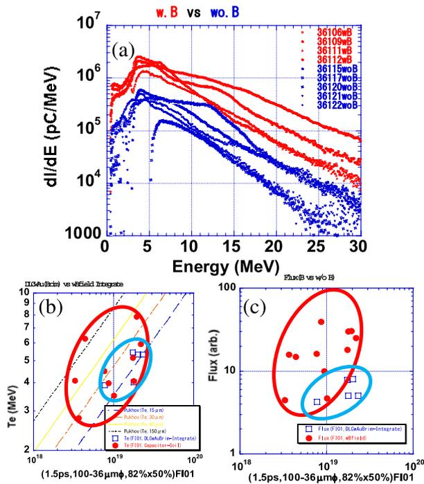
Fig. 4 ESM data with and without  $B_{\text{ext}}$ .  $B_{\text{ext}}$  is induced by the laser irradiation to the parallel plates. (a) Hot electron spectra with and without  $B_{\text{ext}}$ , (b) The laser intensity dependence of  $T_{\text{eff}}$ , (c) The laser intensity dependence of the hot electron flux.
