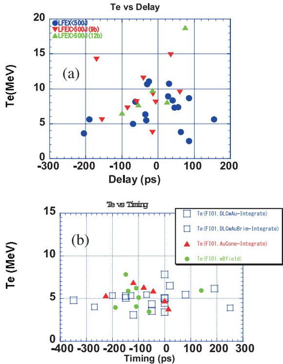
Fig. 3 The implosion timing dependence of  $T_{\text{eff}}$ . The horizontal axis means the deviation between the maximum compression time of the core and the LFEX injection time. (a) in FG02, (b) in FI01.
