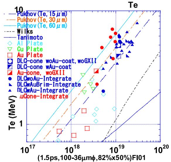
Fig. 2  $T_{\text{eff}}$  in FI01.  $T_{\text{eff}}$  can be obtained from the slope of the hot electron spectrum. Open, half open and closed symbols show the plain, the cone-only and the integrated targets, respectively. Tanimoto and Wilks scalings come from reference [15, 16].
