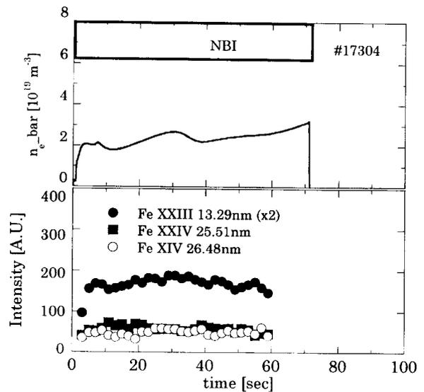
Fig. 6 (a) Time evolution of  $n_e$ , (b) Time evolution of line intensity from highly-ionized iron at the core or the middle on long-pulse NBI discharge.
