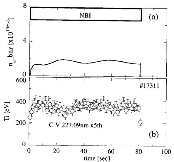
Fig. 5 (a) Time evolution of  $n_e$ , (b) Time evolution of  $T_i$  from C V on long-pulse NBI discharge.
