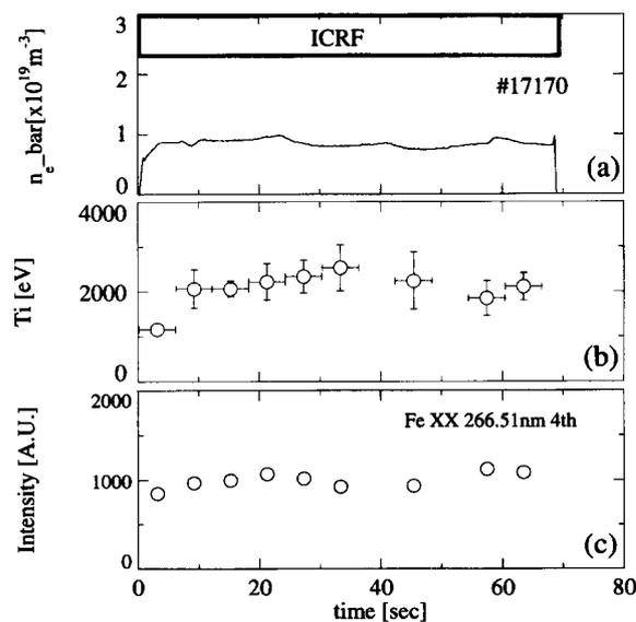
Fig. 2 (a) Time evolution of line-average electron density  $\bar{n}_e$ , (b) Time evolution of Doppler ion temperature  $T_i$  from Fe XX, (c) Time evolution of line intensity of Fe XX spectrum in long-pulse ICH discharge.
