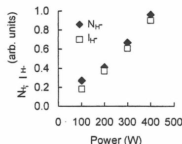
Fig. 3.  $H^-$  ions densities in the source and extracted  $H^-$  current versus discharge power.
