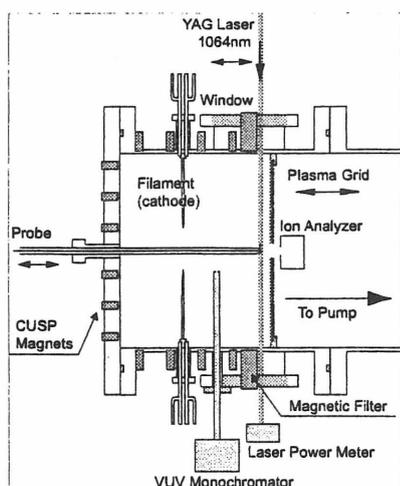
Fig. 1. A schematic diagram of the ion source.
