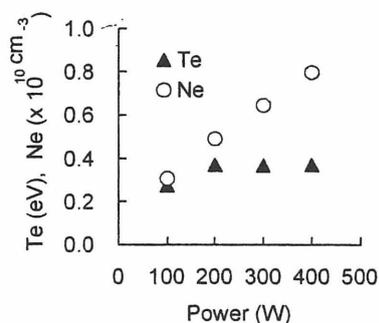
Fig. 2. Plasma parameters ( $n_e$  and  $T_e$ ) versus discharge powers.
