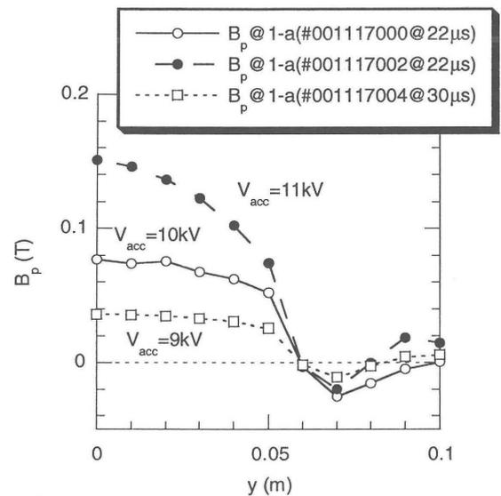
Fig. 2. Radial profiles of the poloidal magnetic field in CTs generated with the charging voltage of 9 kV (open squares), 10 kV (open circles), and 11 kV (closed circles). These profiles are measured at 0.2 m from the exit of the acceleration electrode ( $x = 1.37 \text{ m}$  in Fig. 1).
