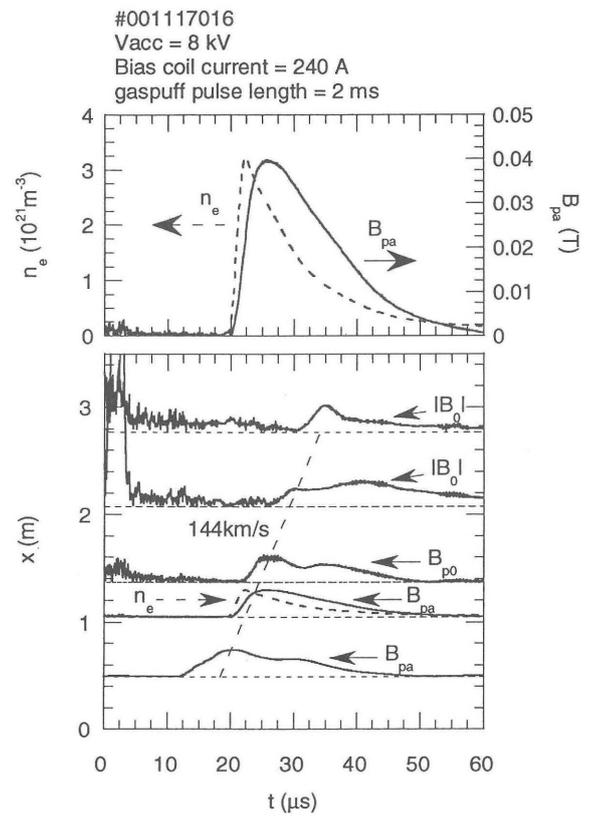
Fig. 1. Waveforms of the electron density  $n_e$ , the poloidal magnetic field strength at the plasma edge  $B_{pa}$  (top) and magnetic signals at various axial locations (bottom). In the bottom figure, each trace is offset vertically by a distance proportional to the axial location, and the broken line denotes the linear trajectory of a CT having 144km/s of velocity.
