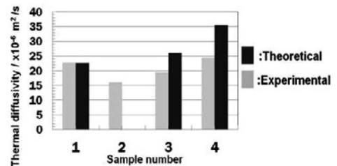
Fig. 3 Thermal diffusivities of samples 1: Fe (SCM440), 2: Fe w/ MWCNT-0.6mg, 3: Fe w/ Cu-0.2mm plate, and Fe w/ Cu-1mm plate.
