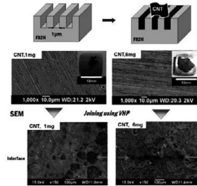
Fig. 2 Procedure of sample preparation for Fe-CNT composite and SEM images of joint surface.
