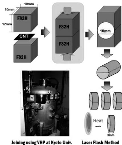
Fig.1 Schematic for the joining procedure of Fe-based composite materials with using VHP.
