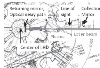
Fig. 2. Geometry of new collection optics (top view).
