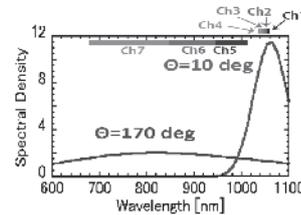
Fig. 1. Difference of Thomson scattering spectra of 10 keV plasma measured by forward (10 deg.) and back (170 deg.) scatterings.
