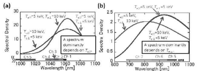
Fig. 3. Example of spectra; (a) forward scattering, (b) backscattering.
