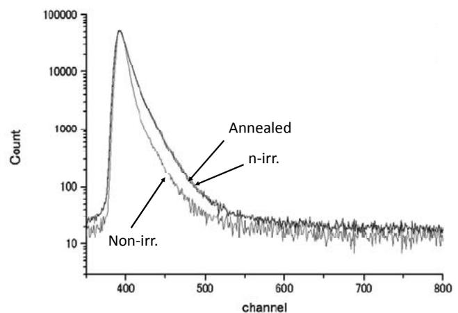
Fig. 1 Positron lifetime spectra of non-irradiated (non-irr.), neutron-irradiated (n-irr.) and annealed (Annealed) specimens. The horizontal axis is channel number corresponding to the time difference between the  $\gamma$ -ray emissions and the vertical axis shows the  $\gamma$ -ray intensity.
