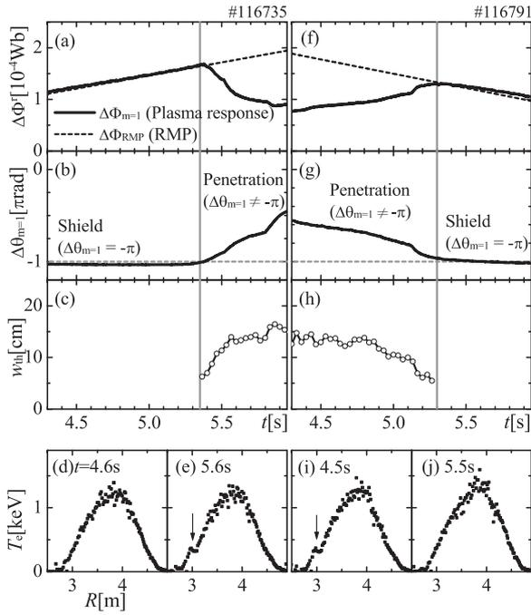
Fig. 2 Time evolution of (a, f) plasma response field (solid) and RMP (dashed), (b, g) phase shift  $\Delta\theta$ , (c, h) flattening width of  $T_e$ , and (c, d, g, h)  $T_e$  profile. (Left) Case of RMP ramp up. (Right) Case of RMP ramp down.
