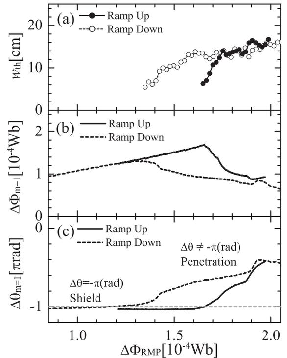
Fig. 3 Trajectories of (a)  $w_{th}$ , (b)  $\Delta\Phi_{m=1}$  and (c)  $\Delta\theta_{m=1}$  with respect to  $\Delta\Phi_{RMP}$ . Solid and dashed lines indicate RMP ramp up case and ramp down case, respectively.
