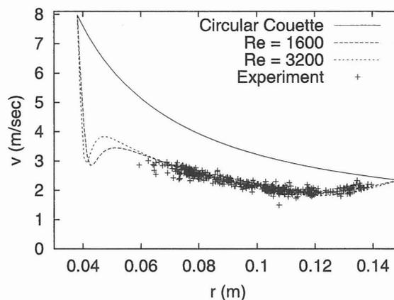
Figure 1: Comparison of azimuthal flow profiles obtained by simulation and experiment.
